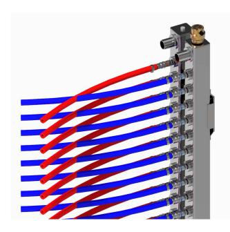
In addition, components used to seal each junction, hoses used for fluids, and couplings must be compatible with the selected wetted material. If they're incompatible, seals could begin degrading, with small pieces breaking off, entering the flow stream, and damaging the downstream heat sinks.
