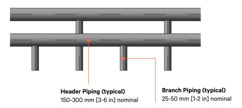
Underfloor designs for piping should leave adequate space for piping, insulation, and pipe crossover. Dimension will vary from site to site.
