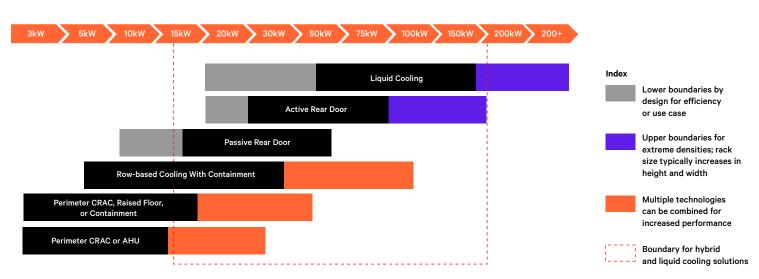
Liquid-cooled systems are often used with air-cooling systems to cool racks at higher densities.
